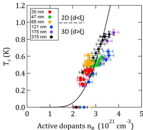
Fig 1: b) Superconducting critical temperature vs active B concentration of thin SiB layers 30 to 175 nm thick, superposed to the theoretical expectations (theory adapted from Boeri, PRL 2004)
