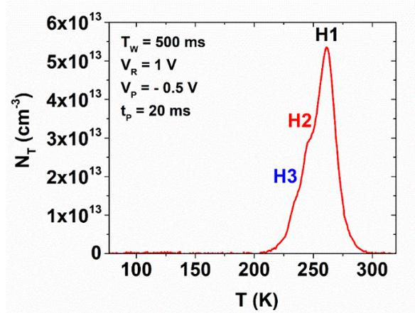
Figure 1: Capacitance DLTS spectrum of the fully depleted silicon-on-insulator transistors. The detection of three hole traps labeled H1, H2 and H3 reveals the presence of electrically active defects in the probed zone located in the onset of the implanted regions.
