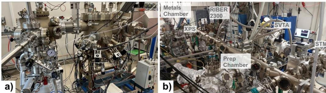
**Fig 1 a)** Arsenides MBE: a modified RIBER C21 designed for both RHEED and grazing-incidence fast atom diffraction measurements, currently used for the growth of GaAs/AlAs, InAs/GaAs quantum dot devices, **b)** Chalcogenides MBE cluster : equipped for the growth of transition metal dichalcogenides, II-VI, III-VI and IV-VI materials (selenides and tellurides).
