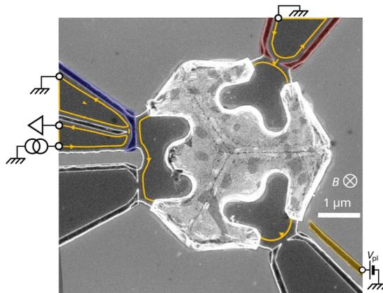
Fig.1. Metal-semiconductor charge Kondo device with a charge sensor to measure entropy.
