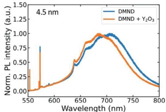
Emission spectrum of NV<sup>-</sup> centers implanted at a depth of 4.5 nm in diamond (blue). Deposition of a Y<sub>2</sub>O<sub>3</sub> thin film preserves emission properties (orange).
