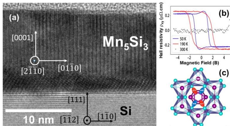
**Fig. 1:** (a) High-Resolution TEM cross-section of a 13-nm thick  $\text{Mn}_5\text{Si}_3$  thin film grown on Si(111). (b) Anomalous Hall resistivity in the antiferromagnetic phase measured at 50 K, 190 K and 300 K. (c) Magnetic and crystalline structure of  $\text{Mn}_5\text{Si}_3$ .
